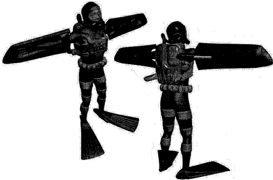
Figure 4 Human exoskeleton for biomimetic propulsion (Neuhaus et al. 2004). The human diver is envisioned to swim by flapping motion, which is similar to the propulsive strokes of certain fish, penguins, and sea lions. Drawing courtesy of P. D. Neuhaus.
